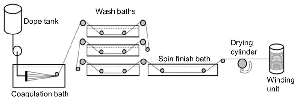
**Figure 4.** Illustration of a wet spinning process.
